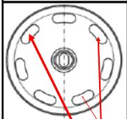
Hole pattern allows for 3 screws securely into the stud
