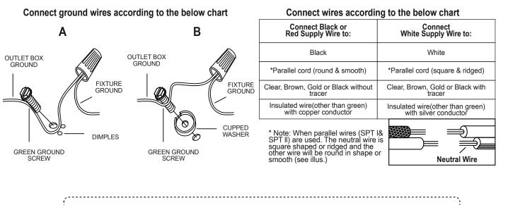
Twist wires together with plastic wire connectors until tightly joined. Wrap each connector with approved electrical tape and be sure that no wire strands are exposed. Carefully tuck all wires into the outlet box.
