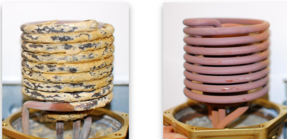
Figure 3. Untreated Element (Left) and Treated Elements (Right)
