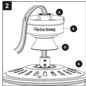
3. Slide the downrod (A) into the yoke of the motor assembly (G), align the holes, then re-install the downrod pin (B) and downrod clip (C). Secure with set screws (U).
