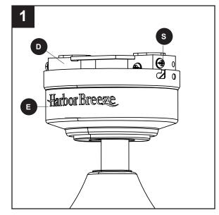
Secure the canopy (E) with the mounting bracket screws (S) previously removed (Step 4, page 8).
