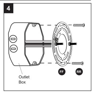
Loosen the ground screw preassembled to the mounting bracket (FF). Wrap the green/bare (ground) supply wire from the outlet box around the ground screw. Tighten the ground screw to secure the ground wire.
