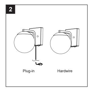
To remove the wall plate (E) from the back of the fixture (A), unscrew and remove the two screw caps (C) from the front of the fixture (A). The wall plate (E) will not be used for hardwire installation.
