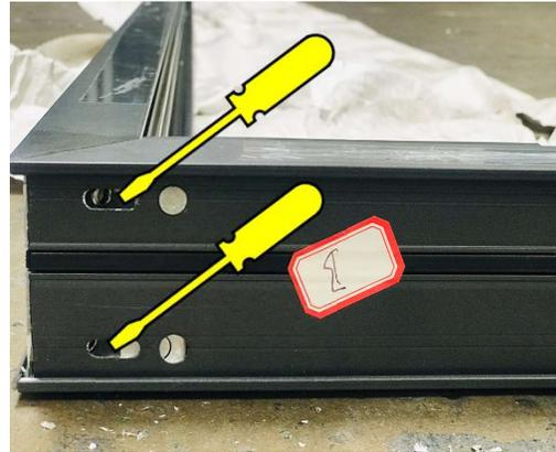
2. Insert the brackets into the frame and make sure the pin gets into the hole.
