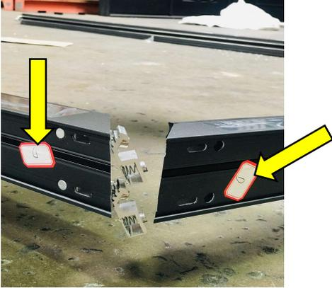
3. Tighten the brackets screws equally until there is no gap between frames.
