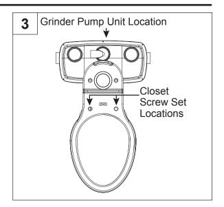
4. Lightly mark the wall with the height of the grinder/tank unit and the bottom and sides of the toilet tank to prevent interference from pipe runs during pipe installation. Remove the toilet from the grinder/tank unit and set it aside until piping is installed.
