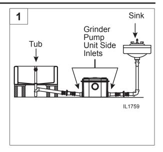
2. Additional fixtures can be attached either to the 2 in. MPT (outside diameter) or the 1½ in. slip (inside diameter). These side inlets are sealed by the factory to prevent leaks when inlets are not used. Before use, these side inlets must be drilled out using a 1¾ in. hole saw.
