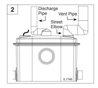
3. A 2 in. x 1 in. 90° discharge fitting and a 1-1/2 in. street elbow vent fitting have been provided for space constraints in an exposed configuration. However, these are not required for a hidden (behind a wall) installation. On a hidden installation, simplify installation and improve performance by replacing the 90° discharge fitting with a straight discharge pipe instead. Use a 2 in. straight coupling and reduce it down to 1 in.
