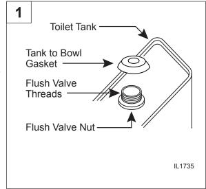
2. Lift the toilet tank right side up and position the tank on the bowl by centering the gasket and aligning holes on the bowl. Install tank to bowl bolts and rubber washers with narrow side down, through the tank and bowl.
