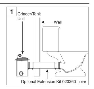
2. Level grinder/tank unit to within 1/8 in. for length and width. Use hydraulic cement or similar material for leveling.
