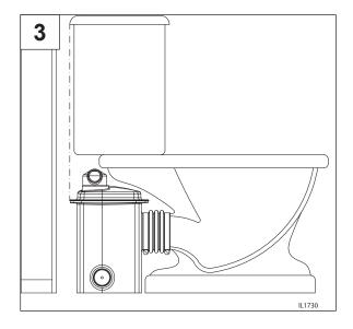
4. Hidden Installation (grinder/tank unit is hidden behind wall). For installation behind a wall, extension kit 023260 (sold separately) is required.
