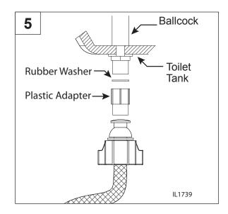
Open the water supply valve and check for leaks. The toilet tank should fill to the proper level. Adjust if required.
