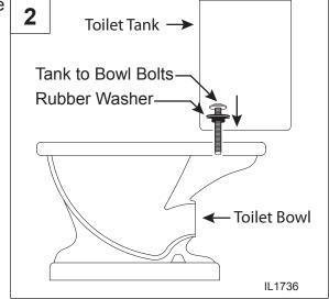
3. Push down on the top of the toilet tank one side at a time while tightening plastic washers and nuts under the bowl. Alternate tightening nuts to achieve a watertight seal, while make sure the bowl and tank are level.
