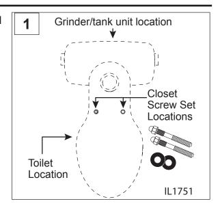
2. Place the toilet assembly over the closet screw sets. Install the anchoring hardware and tighten in an alternating pattern. Check for level and shim as required. Be careful when tightening bolts or nuts against china to avoid cracking the china.
