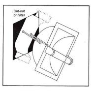
2) Put the Mounting Back-Plate through the hole on wall by tilting it to one side as necessary.
