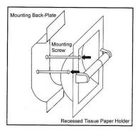
Attach Mounting Back-Plate to the Tissue Paper Holder with the screws (provided). Screw just couple turns to link up these 2 parts. Do not tighten yet.
