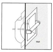
4) At last, tighten up the screws all the way down until Back-Plate is firmly pressed against the inside of the wall to secure the Tissue Paper Holder in position.
