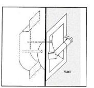
Then, position the Tissue Paper Holder up-right with the side edges well covering the wall hole. Hold firmly against the wall.
