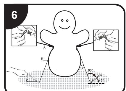
For maximum stability, bring tether down to a 45-degree angle from the inflatable as shown in the illustration. In order to achieve this you may need to wrap the excess tether around the top of the stake.
