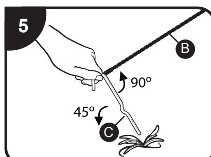
Drive the stakes (C) into ground at a 45-degree angle.
