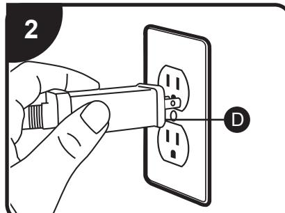
Connect CUL- Listed power supply (D) into connection of fan, plug power supply into standard wall outlet.
