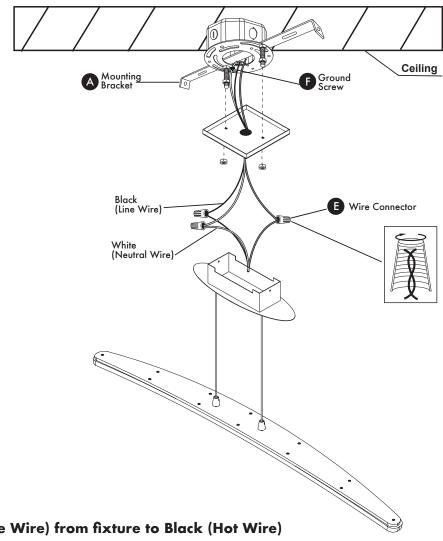
Connect Black (Line Wire) from fixture to Black (Hot Wire) from outlet box.
