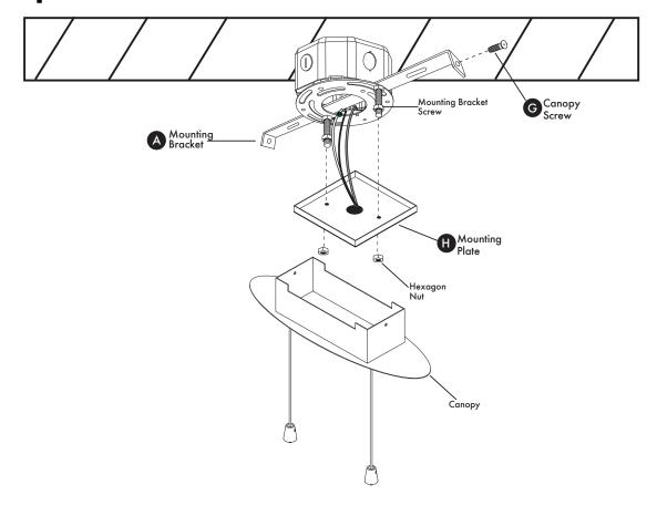
Allign mounting plate (H) to mounting bracket screws. Secure mounting plate (H) with hexagon nuts. Attach canopy to mounting bracket (A). Secure canopy with canopy screws (G).
