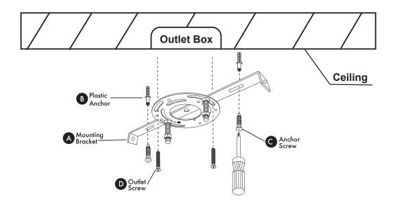
Attach mounting bracket (A) to outlet box with outlet screws (D). Screw anchor screws (C) into plastic anchors (B) to secure canopy cover (A).
