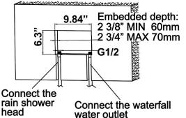
4. The pre-embedded body is supported by hand and installed on the four explosion bolts.
