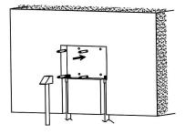
5. Rely on the spirit level to adjust the embedded main body on the horizontal line, use a sleeve to lock the 4 nuts to fix the embedded main body on the wall.
