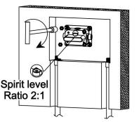
6. Put 1/2 flat spacer into the pre-embedded main body and tighten the water inlet joint.
