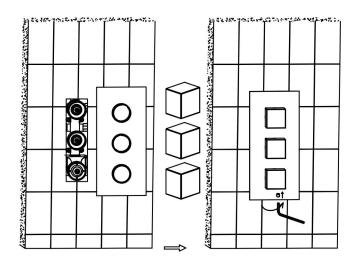
8. Connect all the pipes to check leakage, confirm no leak occurs when turn on water.
