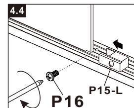
During installing the glass and the blocks(P15), be careful to avoid collision between the glass corners and the ground,which may cause the glass to break.
