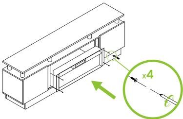
Fix the appliance to the TV stand with 4 silver screws according to the hole position.
