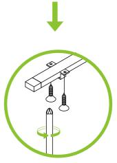
Hold the light strip with the clip and lock the screw.
