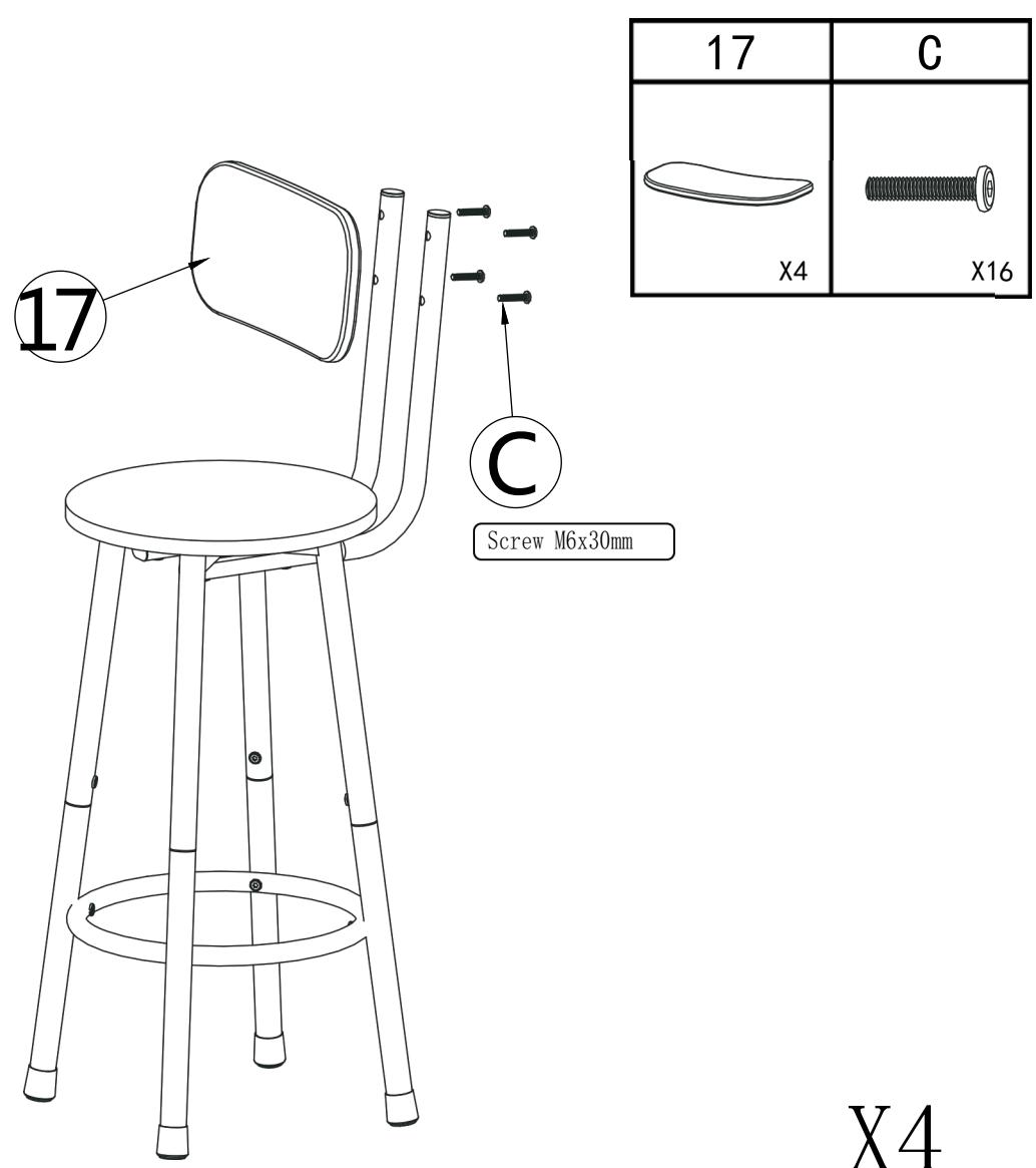
EN-During the assembly, please first half-tighten all the screws into the holes.
