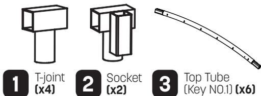
Insert **four key no. 1 top tubes (3)** into **four T-joints**, and **two key no. 1 top tubes** into **two sockets**. **Make sure the holes in the tubes face the ground!**
