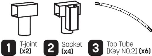
Insert **two** key no. 2 top tubes (**3**) into **two** T-joints, and **four** key no. 2 top tubes into **four** sockets. **Make sure the holes in the tubes face the ground!**
