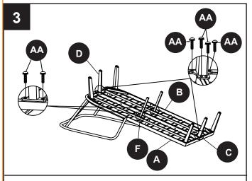
Hand tighten AA. Do not tighten with wrench, DD, until all bolts have
