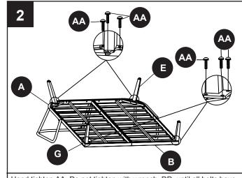
Hand tighten AA. Do not tighten with wrench, DD, until all bolts have been installed.
