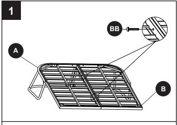
Hand tighten BB. Do not tighten with wrench, DD, until all bolts have been installed.
