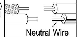
**Twist wires together with plastic wire connectors until tightly joined, and wrap each connector with approved electrical tape. Be sure that no wire strands are exposed and then carefully tuck all wires into the outlet box.**
