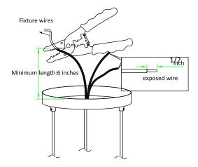
6 » Carefully pass supply wires through mounting plate assembly (A).
