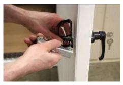
(159) Attach L-handle as shown using a 5/32 Allan Wrench. Adjust as needed.
