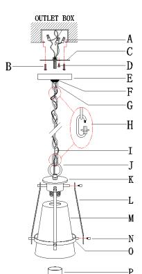
Step A1: Connect the socket cup (K) to the iron hoop (O) with a flat iron bar (L) and fix it with screws (N).
