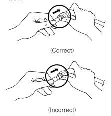
2) Pull the tube to make sure that the tube is tightly fastened and then insert the clip.
