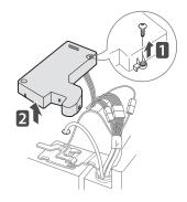
3 Remove the cover and pull out the tube **1**. Disconnect all wire harnesses **2**.
