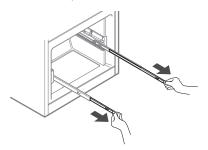
2 Grasp the drawer on each side and hook the drawer supports into the rail tabs located on both sides.
