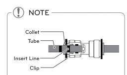
Gently press the Collet and insert the tube until only one line shows on the tube.
