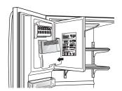
2 Avoid touching the auto shutoff (feeler arm) when replacing the ice bin. See the label on the ice compartment door for details.
