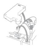
5 Hold the water supply connection and gently push in the collet to connect the water supply line as shown in 1 and 2. Insert the tube at least 5/8 inch (15 mm) into the connector. Assemble the clip to the joint part for fastening.
