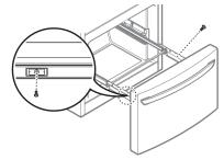
4 Grip both sides of the drawer and pull it up to remove it from the rails.
