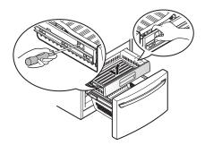
3 Remove the screws from the rails at both ends.
