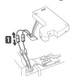
3 Rotate the hinge lever 1 clockwise. Lift the top hinge 2 free of the hinge lever latch.
