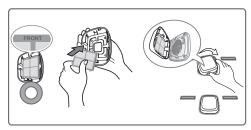
After changing the filter, push and hold the Air Filter button for three seconds to reset the filter sensor.
