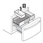
On the left rail, use a flat blade screwdriver to push in on the tab to release the drawer from the rail, as shown below. Once the left side is loose, push the tab on the right side with your finger to release the drawer. Lift the front of the drawer up, then pull it straight out.
