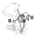
A Rotate the hinge lever counterclockwise
