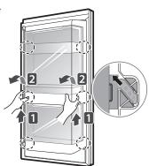
2 To replace the Door-In-Door case, line the tabs on the Door-In-Door Case with the slots on the door and push down until it snaps into place.
