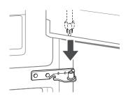
2 Fit the hinge 1 over the hinge lever latch and slot it into place. Rotate the lever 2 counterclockwise to secure the hinge.
