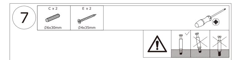
Insert wooden dowel(C) into plate 6 at first, then connect with the two components. Fix plate 5 to plate 6 with screw(E) as shown.
