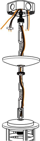
Pull the supply wires with ground wire through the chain alternate links.
