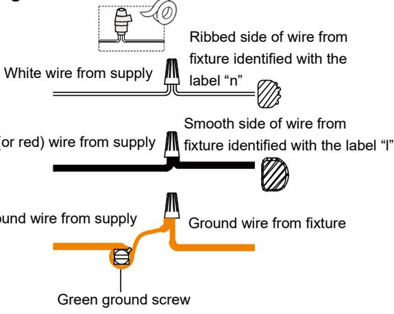
Ribbed side of wire from fixture identified with the label "n"
