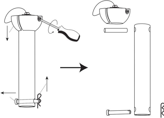
② Pass the cable through the down rod and lock the down rod.
