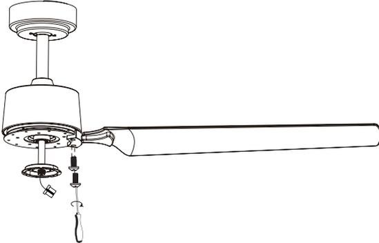
② Remove the pre-installed screws.
