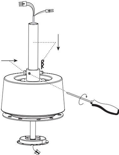
③ Install the Yoke cover and Canopy. Then insert the fixing pin, push the Hanging ball up, and fix it with screws.
