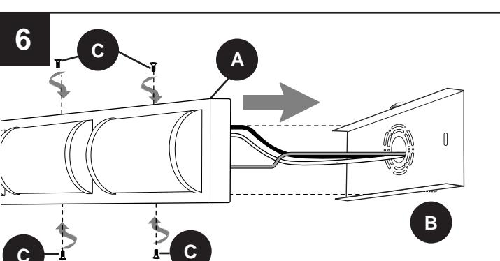
Before tightening C completely, use level (not included) to check A -- adjust if necessary.
