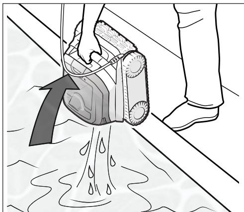
Figure 6. Always Remove Cleaner Using the Handle
