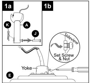
Insert downrod (A) through yoke cover (D) and canopy (C). Thread wires from motor housing (E) up through downrod (A).
