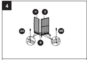
Once all connections are made, tighten AA with hand.
