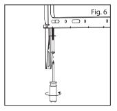
**IMPORTANT!** The safety screws must be tightened at all times to prevent the display from being accidentally knocked from the mount.
