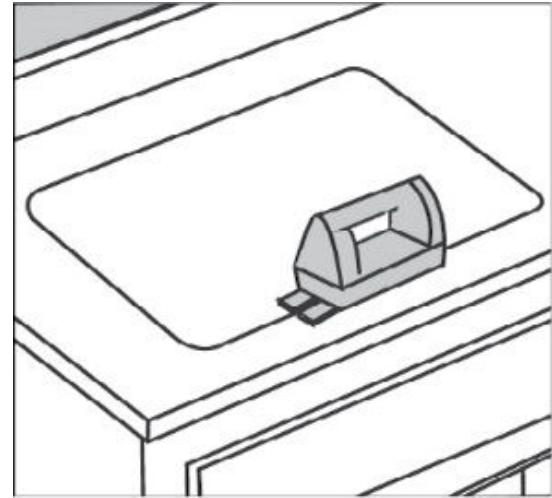
**1** Check the cut-out template against the actual sink to ensure a proper sized cut-out, then Place the cut-out template in the desired location on the countertop
