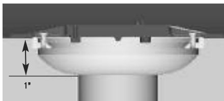
Fig. 7: Support Plate Aligned Over Screw Holes
