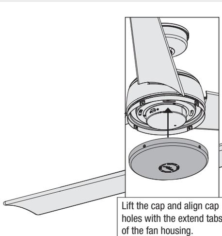
Lift the cap and align cap holes with the extend tabs of the fan housing.
