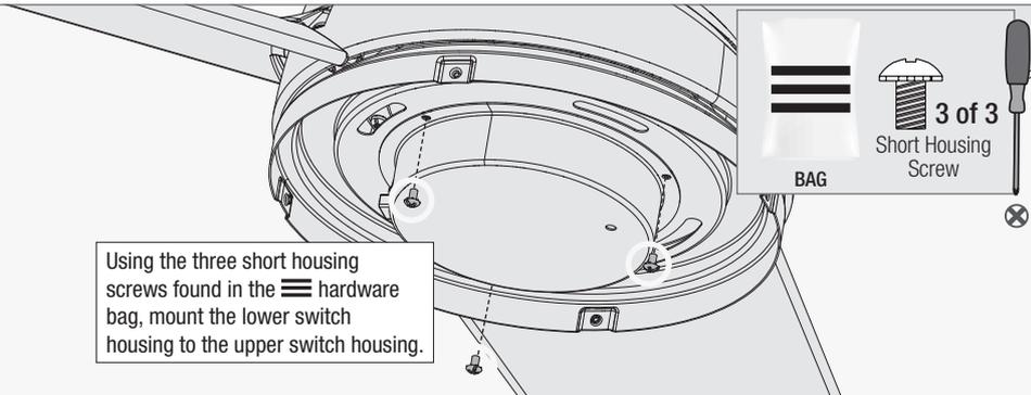
Using the three short housing screws found in the
