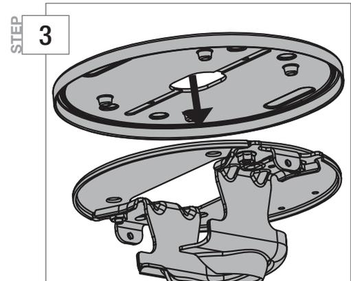
Install the ceiling plate gasket onto the ceiling plate. The four holes in the ceiling plate should lineup with the four posts in the gasket.
