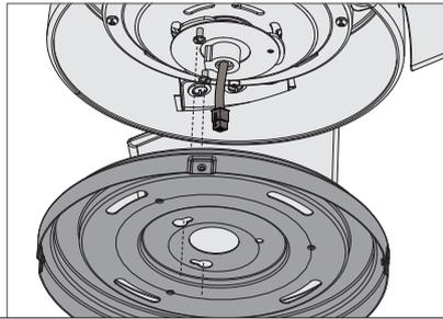
Feed the wire plug through the center hole of the upper switch housing. Align the keyhole slots in the upper switch housing with the two screws you just installed. Lift the upper switch housing so that the keyhole slots engage the two screws, and twist counterclockwise to lock the upper switch housing into place.
