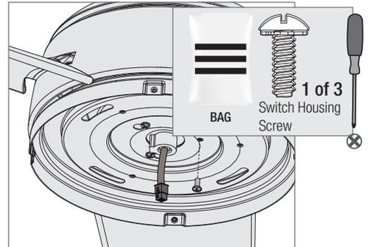
Insert the third screw found in the
