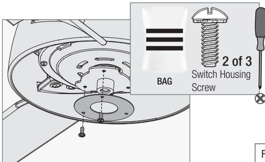
Partially install two switch housing screws, found in the
