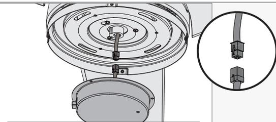
Lift the the lower switch housing and connect the plugs. Make sure to line up the colored markings on the connectors and that the connectors latch.
