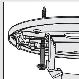
Use the wood screw to poke holes through the rubber gasket in order to install the ceiling bracket assembly to your support structure or ceiling fan-rated outlet box.
