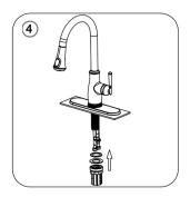
4. Install the rubber washer, metal washer, and quick nut onto the faucet shank in that order underneath the countertop. Tighten down the quick nutensuring the faucet is in the proper position.
