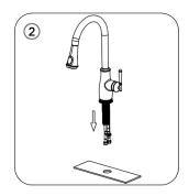
2. For single hole installation insert the hot and cold supply lines and shank through the hole in the countertop.
