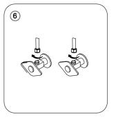
6. Connect the open ends of the hot and cold supply lines to the shut off vales. Ensure the faucet is in the off position and turn on shut off valves. Check for leaks.
