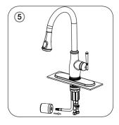
5. Install the gravity weight onto the spray hose, take the open end of the hose and connect it to the quick connection at the base of the faucet shank. The weight should be placed approximately 2" above the natural curve in the hose.
