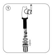
1. Remove the quick nut, metal washer and rubber washer from the faucet shank.
