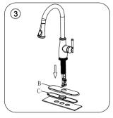
3. For a 3-hole installation insert the base plate panel into the base plate and slide it onto the faucet shank. Insert the hot and cold supply lines, spray hose and shank through the hole in the countertop.
