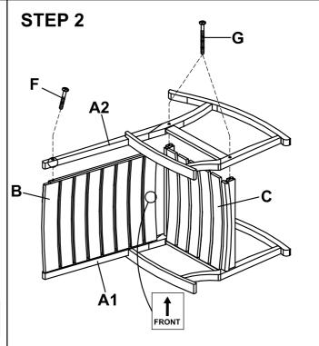
Install Back support (B) and Seat (C) into corresponding holes of Right side frame (A1). Attach the Left side frame (A2) onto Back support (B) and Seat (C). Secure Left side frame (A2) using 1" Bolt (F) and 1 1/2" Bolts (G), as shown.
