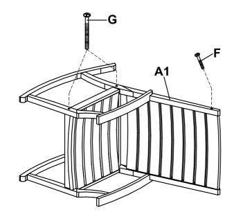
Invert the Rocker and repeat the step 2 procedure to secure the Right Side frame (A1).
