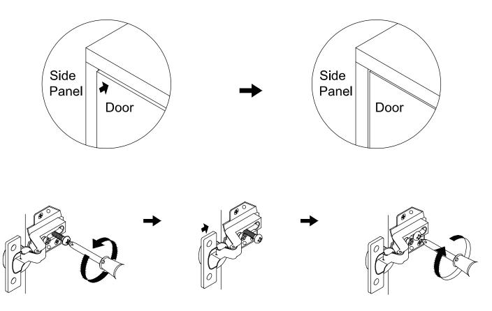
If the top of the door is not level with the side panel, loosen the screw at the back of the hinge as shown, then move the hinge in or out until the desired gap is achieved, and then re-tighten the back screw.
