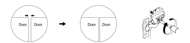
If the gap is too tight between the two doors, loosen the screw at the front of the hinge as shown to make the adjustment and then re-tighten the screw.
