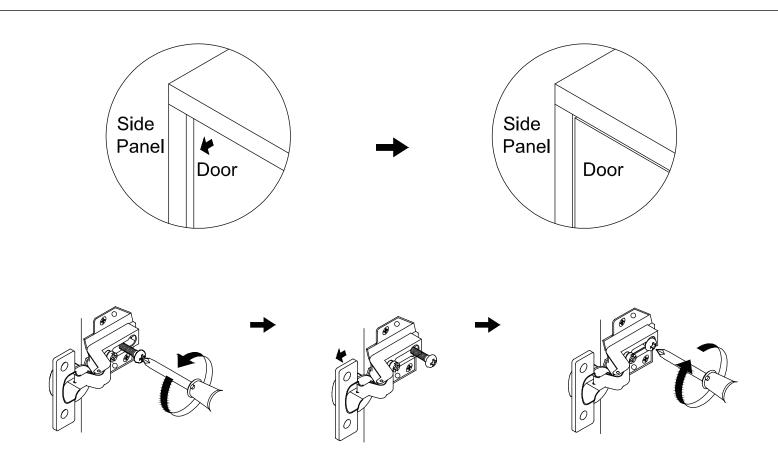
If the top of the door is not level with the side panel, loosen the screw at the back of the hinge as shown, then move the hinge in or out until the desired gap is achieved, and then re-tighten the back screw as shown.
