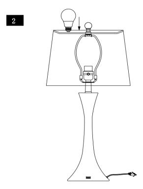
Step 2 Insert the bulb(G) into the socket(C).
