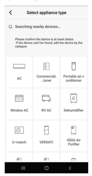
7. Follow the on-screen prompts to connect the unit. After pairing the unit with the app, you will be prompted for the Wi-Fi network to be used with the unit. Select the proper Wi-Fi network ID and enter the network password. Please note the unit is not compatible with 5 GHz networks.
