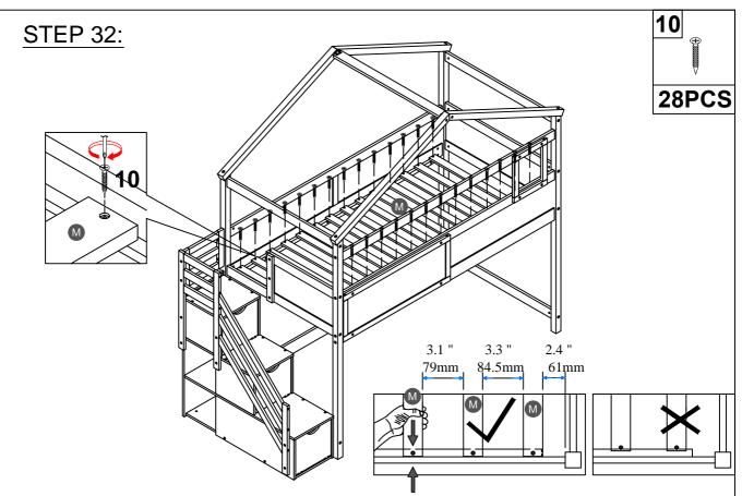
**NOTE:** Please make sure the bed slats close to the side rail before locking the screws to avoid breakage. This step is required for both the left and right sides. Moreover, please do not lock the screws of the bed slats at the outermost edge to avoid damaging.
