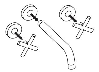
6. Attach the spout to the valve by twisting it into the middle valve outlet. Apply plumber's tape or a small amount of thread sealant to the threads before attaching.
