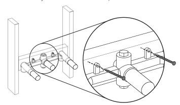
3. Attach your existing water lines to the valve. Apply thread sealant or plumber's tape to the threaded connection to ensure a watertight seal.
