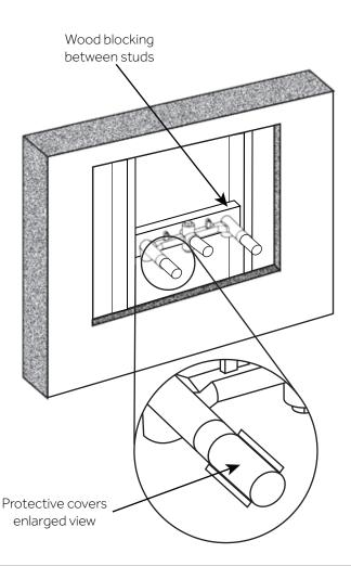
2. Mount the rough-in valve into its prepared location. Attach the valve body using the provided hardware. Use a level to ensure that the valve is mounted completely level.
