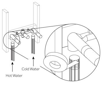
4. Once your finished wall has been completed, remove the protective plastic sleeves from the valve. Remove the plug from the spout outlet using a 14mm socket wrench.
