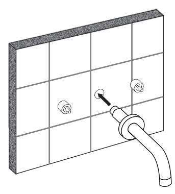
7. Attach the hot and cold handles by sliding them onto the left and right stems. Secure each handle by tightening the set screw on the bottom of the handle, using the provided hex wrench.
