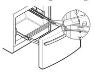
3 Lower door into final position and tighten the screws.
