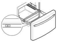
4 With the drawer pulled out to full extension, insert the lower basket in the rail assembly.
