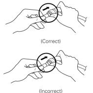
Pull the tube to make sure that the tube is tightly fastened and then insert the clip.
