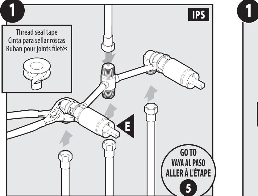
This valve (E) can be plumbed using threaded connections (IPS). The water inlets, the outlets to the tub spout and to the showerhead are  $\frac{1}{2}$ " male pipe thread. Use thread seal tape when making these connections. Wrap the tape onto the threads in the same direction the adapter will thread on. Use adjustable pliers or a pipe wrench to hold the valve body when tightening the connections. Go to **step 5**.
