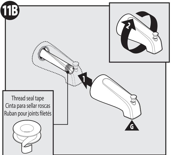
IPS (threaded) spouts are designed to screw onto a pipe with 1/2 inch male pipe threads. To determine the proper pipe length, measure from the inside elbow shoulder to the wall (y) and from the threaded adapter inside of the tub spout to the base of the tub spout (x), then add 1/4". Place thread seal tape around the pipe threading and a sealant (plumbers putty or caulk) around the base of the pipe to prevent leaking behind the wall. Thread the tub spout onto the pipe until flush with the wall.
