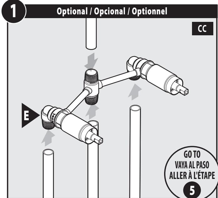
If soldering copper tubing (CC) into valve (E) insert  $\frac{1}{2}$ " copper tubing into the hot and cold water inlets and the shower riser and tub drop outlets. Then, go to **step 5**.
