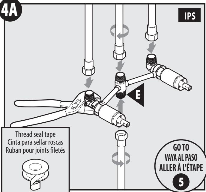
This valve (E) can be plumbed using threaded connections (IPS). The water inlets, the outlets to the tub spout and to the showerhead are  $\frac{1}{2}$ " male pipe thread. Use thread seal tape when making these connections. Wrap the tape onto the threads in the same direction the adapter will thread on. Use adjustable pliers or a pipe wrench to hold the valve body when tightening the connections.
