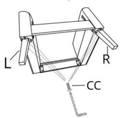
Fix the Back Feet (divide the left and right).
