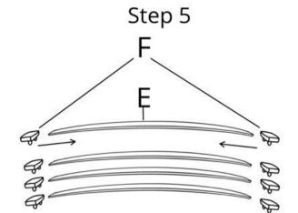
Make sure the convex surface like the bridge is upward and put on the cap.
