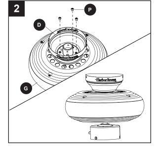
Raise the fan and place the canopy (D) on the hook on the mounting bracket (E), temporarily leaving hands free for the wiring process.
