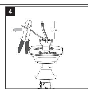
If you decided to cut back the lead wire in Step 4, strip 1/2 in. of insulation from the end of the white wire. Twist the stripped ends of each strand of wire within the insulation with pliers (not included). Repeat this step for black and blue wires.
