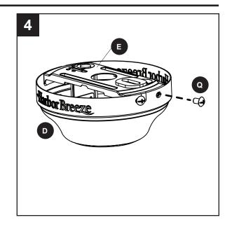
5. Attach mounting bracket (E) to outlet box (not included) using screws and washers provided with the outlet box.
