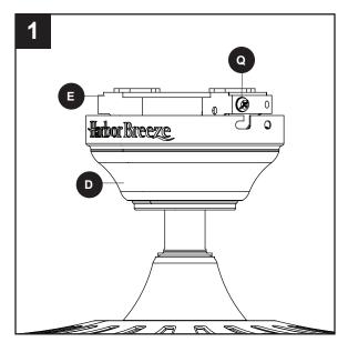
Secure the canopy (D) with the mounting bracket screws (Q) previously removed (Step 4, page 8). Tighten all mounting bracket screws (Q) securely.
