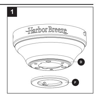
Remove three Phillips-head closemount screws (P) from the top of the motor assembly (G). Align the canopy (D) with the holes in the top of the motor assembly (G), then re-install the Phillips-head closemount screws (P) to secure the canopy (D) to the top of the motor assembly (G).
