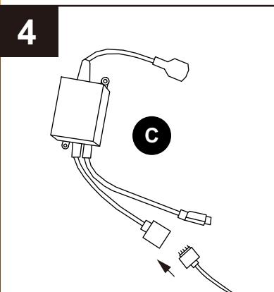
Plug the lead wire from the tape light into the lead wire from the receiver (C).
