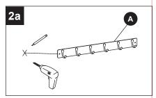
For drywall installations, remove rail (A) and drill 5/16 in. pilot holes at marks. Place anchors (BB) into holes.
