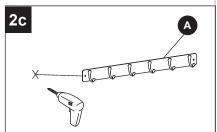
3. Secure rail (A) to mounting surface with screws (AA).
