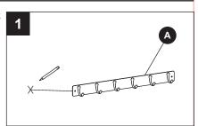
2a. For solid wood/wood stud installations, remove rail (A) and drill 3/32 in. pilot holes at marks.
