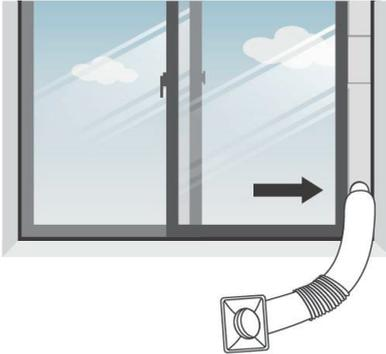
**Step 5:** Attach the hose connector to the exhaust air outlet of unit.
