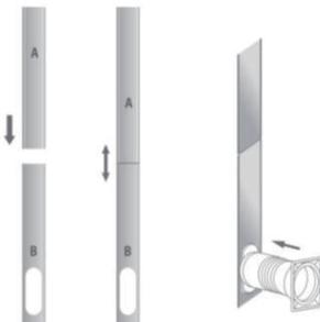
**Step 4:** Close your window to secure the kit in place. It needs to hold the windows kit firmly in place, and secure the window kit with duct tape if required. It is recommended that the gap between the adapter and the sides of the window should be sealed off for maximum efficiency.
