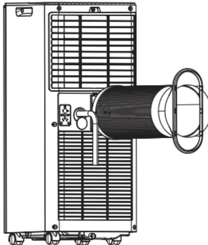
**Step 6:** Adjusting the length of the flexible exhaust hose, to make sure the distance between the unit and the window will be more than 28" , the height from exhaust hose to the floor will be more than 35" . And avoid bends in the hose. Then place AC near an electrical outlet.
