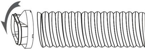
**Step 3:** Extend the adjustable window kit to the length of your window. Connect the exhaust hose to the window kit. Fasten the butterfly nut to fix the exhaust hose and window kit.
