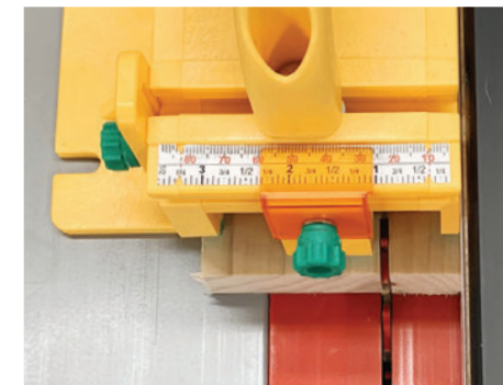
Fig. 4 Grr-ripper SafeRip Cursor with scale
