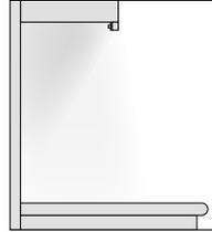
**Continuous run mounting** of LED tape lighting is achieved by drilling a 1/2 in. hole through cabinet side frame lips. When mounting on the back side of the front frame lip, use a multi-tool oscillating saw to make small vertical cuts in the dividers to create slots that allow the tape lighting to pass from one cabinet to another.
