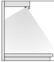
If your countertop is reflective, install the LED tape lighting on the inside back of the cabinet lip frame with the LEDs facing towards your backsplash. This method helps eliminate unwanted light reflections and bright spots reflecting off your countertop. Because of the wide beam angle of the tape light, this mounting position will still provide ample lighting.
