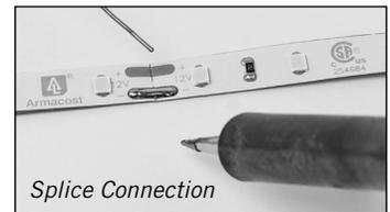
Soldered connections are required for marine and RV applications due to vehicle movement and vibrations.
