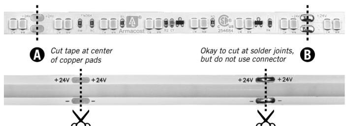
**IMPORTANT:** Always use the + / - indicators printed on the tape light to maintain the same polarity (+ to + and - to -).
