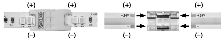
If the + / - marks do not line up, flip the tape and use the opposite end for proper alignment.
