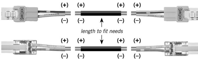
**NOTE:** Be sure all 24-volt connections are secure and protected from electrical shorting. Options include electrical tape, small wire nuts, crimp connectors, etc.
