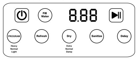
**On/Off Power icon** (**U**)- Powers on the Steam Dryer Closet. All the selections on the Control Panel illuminate.
