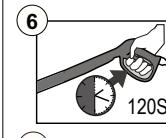
Run water hose for 120 seconds with the motor in OFF position. This helps drain air from the tank and lines.
