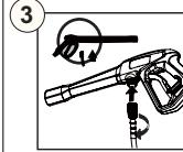
Insert high pressure hose into trigger handle.
