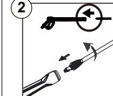
Assemble pressure washer gun to spray wand.
